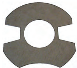
135066 Gasket Servicing: M35J ID 23.00, OD 51.75, Thickness 0.40
