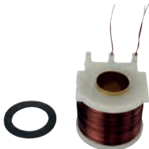
138940 Solenoid Coil 24 V, ID 21.10, OD 46.75, Height 39.00
