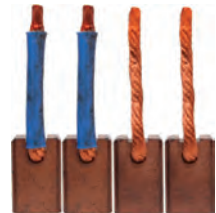
140339 Brush Set Replacing: TAJ111, TAJ103 12 V, Length 22.00, Lead length 43.50, Height 15.00, Thickness 8.00
