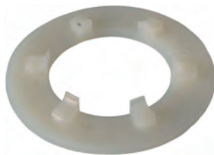
235237 Spring/roller retainer Replacing: 1120591511 Servicing: 0123325500, 0123525501, 0123525504 ID 27.25, OD 45.45, Thickness 1.75, Material Shockproof plastic
