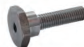
238957 Bolt Servicing: 0001368011, 0001368083 Length/rear collar 41.50, Thread length 29.00, Thread size M5, Thread size/rear M8
