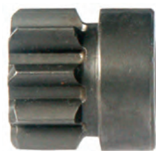
134174# Dp Gear ID 13.00, OD 25.20, Height 25.45, No./teeth 9
