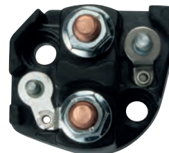
231880 Solenoid Cap Servicing: 63223435, 63223532, 636019063, 636019066, 85541020 OD 50.00, No./terminals 4 w/ 30H terminal. HC-CARGO 137790.
