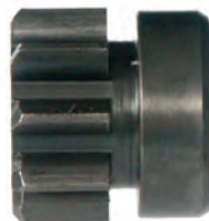
134188 Dp Gear ID 12.00, OD 29.00, Height 26.85, No./teeth 9
