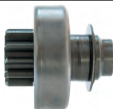
139478 Drive Replacing: 594279, 187528, 059427 Servicing: D7R12, D7R127, D7R19, D7R27, D7R28, D7R281, D7R32, D7RP123 ID 12.00, OD 29.00, OD/housing 54.00, Total length 54.00, Splines A 10, No./teeth 11, Rotation CR
