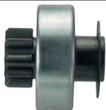
333934 Drive Replacing: 195334, 195041, 194039 ID 12.00, OD 28.30, OD/housing 49.00, Total length 45.20, Splines A 10, No./teeth 9, Drive type Steel, Rotation CR
