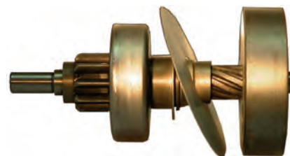
230253# Drive Manufacturer: Valeo Replacing: NE210, 182052 Servicing: D9R121, D9R84 OD 68.80, Total length 129.30, Splines A 9, No./teeth 10, Rotation CR Drive: HC-CARGO 132020.
