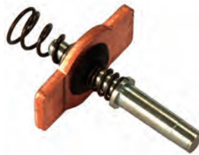
231839 Moving Contact Servicing: 77222 Length 32.00, Shaft measurement 30.00, Thickness 2.50, Width 12.20
