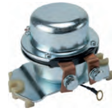
333013 Solenoid 24 V, Intermittent load 1000 Amp., B+ M8, OD 90.00, Total length 133.00, No./terminals 4
