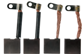
140340 Brush Set Replacing: TAJ102 12 V, Length 14.00, Lead length 33.60, Height 16.00, Thickness 6.00
