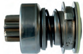
130406 Drive Replacing: TMB420 ID 12.00, OD 26.00, OD/housing 46.15, Total length 68.50, Splines A 10, No./teeth 9, Rotation CR
