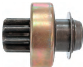
139153 Drive Replacing: 594033, 594030 Servicing: D6RA15, D6RA7 ID 12.00, OD 25.20, OD/housing 48.00, Total length 56.65, Splines A 9, No./teeth 9, Rotation CR
