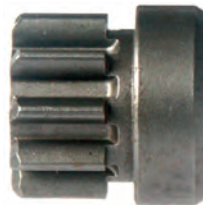
134179 Dp Gear ID 12.00, OD 26.70, Height 27.00, No./teeth 10
