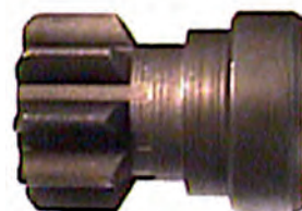
137012# Gear Wheel ID 12.00, OD 25.45, Height 36.40, No./teeth 9
