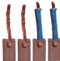
140334 Brush Set Replacing: TAJ100 12 V, Length 18.00, Lead length 33.00, Height 11.00, Thickness 7.00
