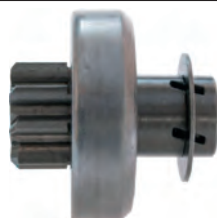
139477 Drive Replacing: NE971, 594345, 187788, 182848 Servicing: 105119C, D7E15, D7E18, D7E19, D7E20, D7E27, D7E38, D7E4, D7E47, D7E6, D7E8, D7ED28, D7EP12 ID 11.00, OD 23.80, OD/housing 46.00, Total length 44.00, Splines A 5, No./teeth 8, Rotation CR Drive: HC-CARGO 139477 can only be used w/ Armature: HC-CARGO 139434.
