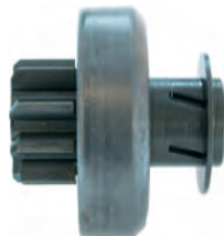
139473 Drive Replacing: NE949, 594287, 492828, 188251, 187996, 187863, 187336 Servicing: D7E1, D7E16, D7E23, D7E26, D7E39, D7E5, D7E52, TS8E6 ID 11.00, OD 25.30, OD/housing 46.00, Total length 41.00, Splines A 5, No./teeth 9, Rotation CR Alternative no.: 335234
